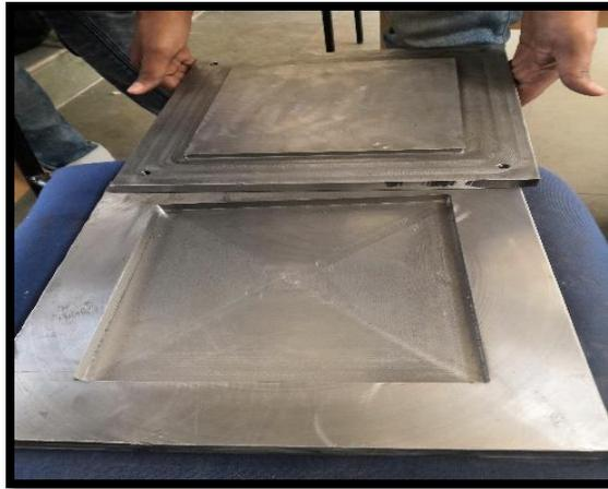
*Figure 1. Mild Steel Mould*
