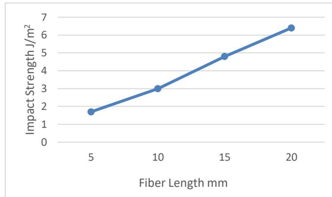
Figure 6. Graph between Impact strength and fiber length
