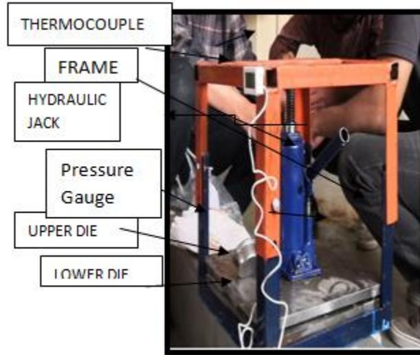
Figure2. Compression Moulding Setup
