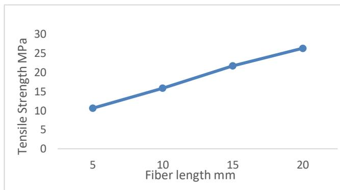
Figure 4. Graph between tensile strength and fiber
