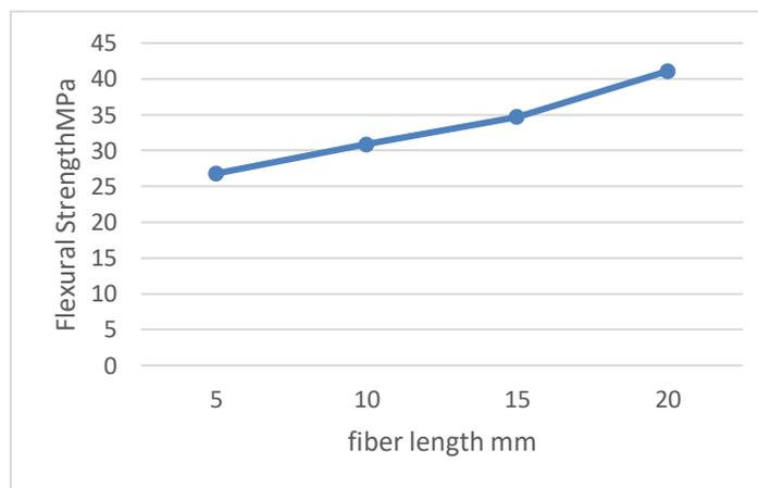
*Figure 5. Graph between flexural strength and fiber length*
